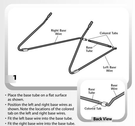
• Make sure both colored tabs on the base wires are visible through the holes in base tube.
